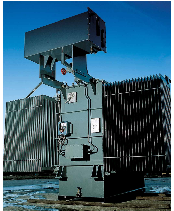
2.5MVA multi-tapped power transformer. Primary voltage 400V, secondary 3.3/6.6/11kV.
